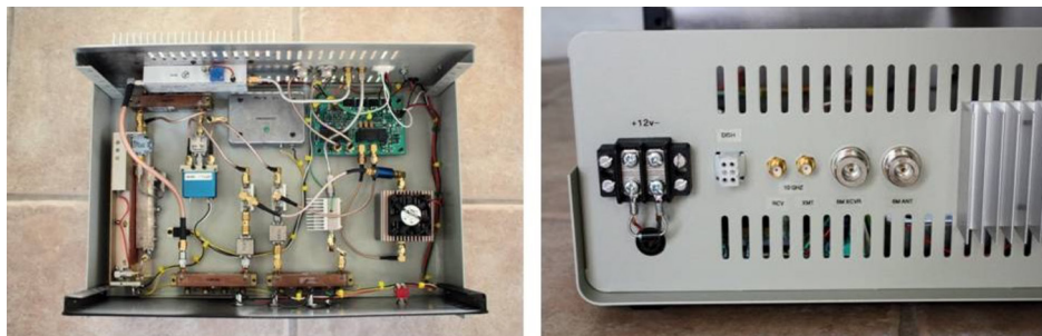
Figure 12: 10W transverter (transmit/receive converter)
