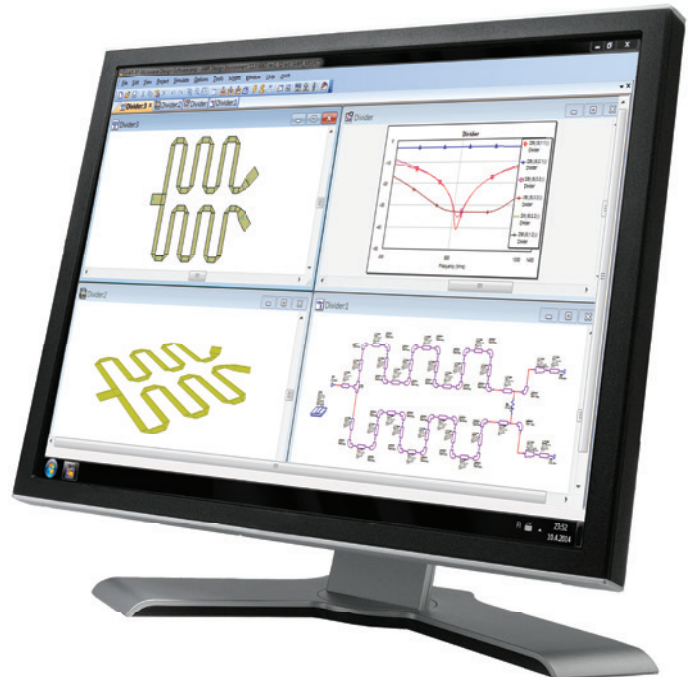
Microwave Office divider design: schematic, layout, and simulation results.
