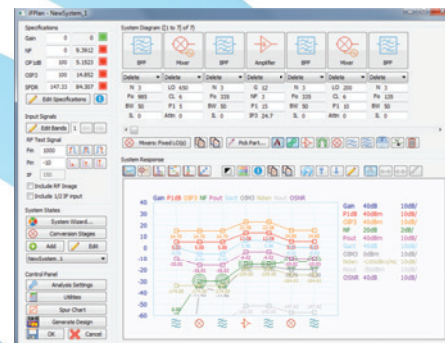
Figure 1. RFP graphic interface with views of the system architecture and access to setup and utilities.
