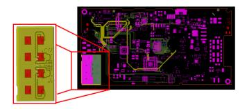
Integrated mmWave IP (antenna array in the red popout) on a mixed-signal PCB
