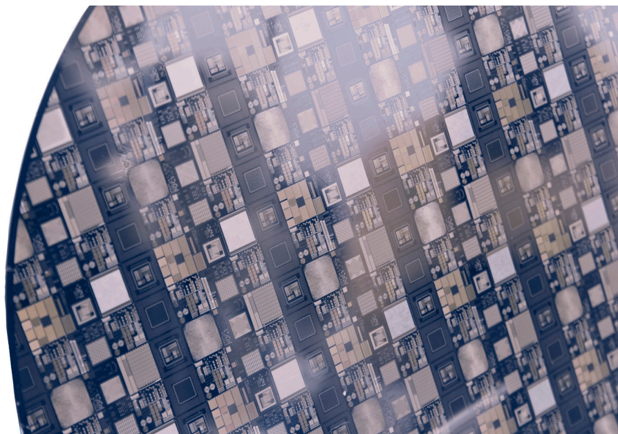
Figure 1: Processed wafer with integrated passive elements
