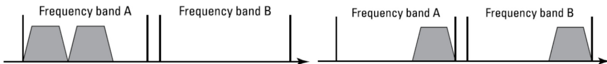
Figure 2: Allocation of the intra-band contiguous (left) and inter-band carriers (right) (image courtesy of Qorvo)
