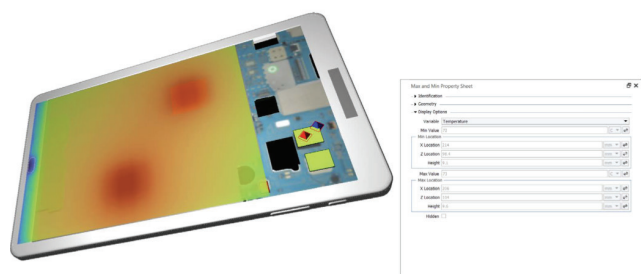
Figure 5: Max and min markers can be placed on a component to show the location and value for the highest and lowest predicted temperature
