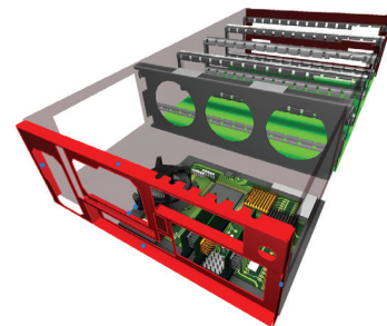
Figure 2: The Celsius EC Solver CAD editor enables users to move, resize, or delete existing features in the geometry
