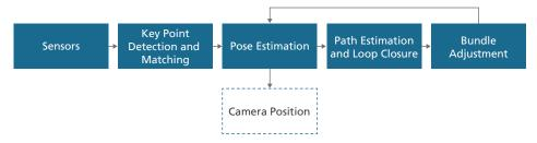
Figure 3: SLAM process flow
