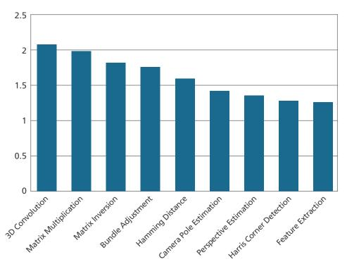
Figure 5: The Vision Q7 DSP speed over the Vision Q6 DSP: Up to 2X improvement on various blocks of SLAM
