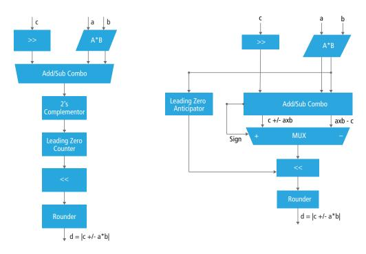
Figure 2: Conventional FMA block diagram
