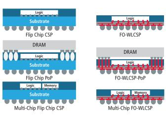
Figure 1: Examples of chip-scale-packaging compared with UT-FOWLCSP
