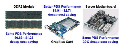
The DDR3 memory module optimization with 36 DRAMs resulted in \$0.69 savings per DIMM. A decap area reduction of 32% also was achieved while maintaining PDS impedance performance and marginally improved power plane noise performance (as shown in **Figure 5**). A high-speed graphics card was optimized for combined PCB-package PDS performance. A multi-domain package-board power plane resonance was reduced to yield significantly improved performance with nearly \$2 in manufacturing cost savings.
