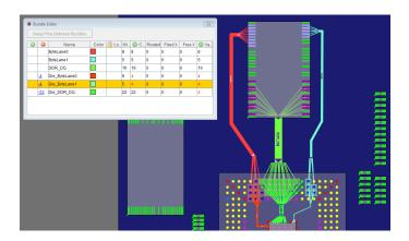
Figure 2: PCB-driven package and die assignment
