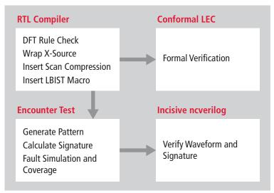
Figure 3: LBIST insertion and validation flow
