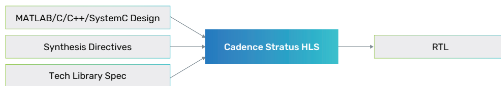
Figure 2: Stratus HLS takes an abstract design description in MATLAB, C, and C++ and optimizes the micro-architecture, yielding more optimal RTL that meets design constraints
