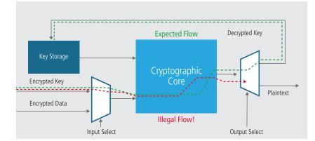
Figure 4: Illegal key flow in customer design detected by Radix
