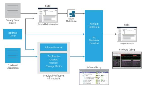
Figure 1: Tortuga Logic and Cadence flow for security verification
